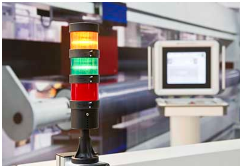
Figure 8: Andon Light System Applied on Equipment
